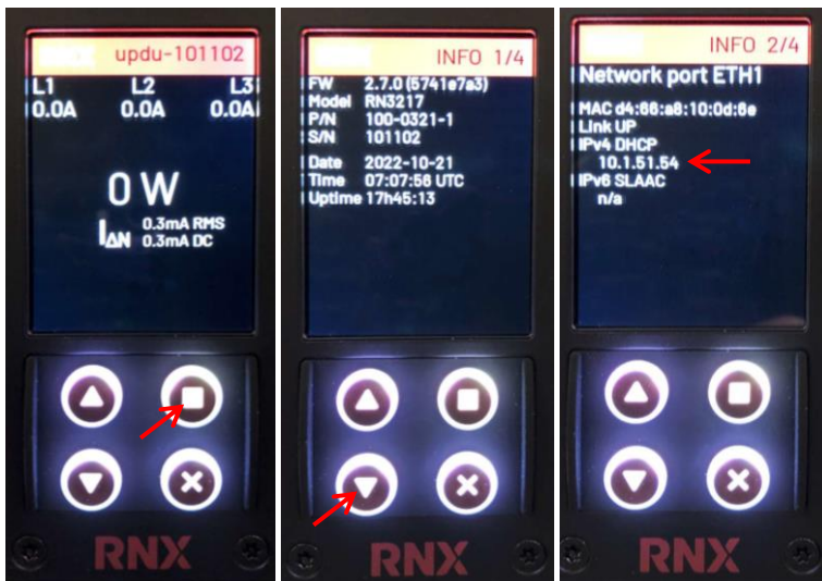
Figure 1: Finding the IP address on the PDU display.
